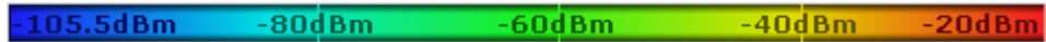
Fig. 4-5: Linear color curve shape = 0; colors are distributed evenly over the complete result range
